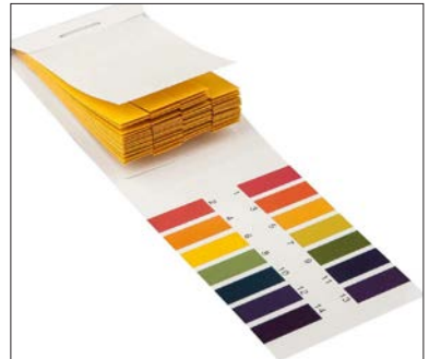
Litmus paper strips from a fish or pet store will give a basic idea of your soil's pH content.
